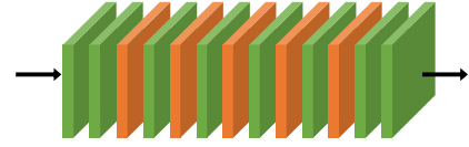
Fig. 3. Structure of \mathcal{V}_k and \mathcal{W}_k CNNs. The green and orange layers denote convolutional and ReLU layers, respectively.
